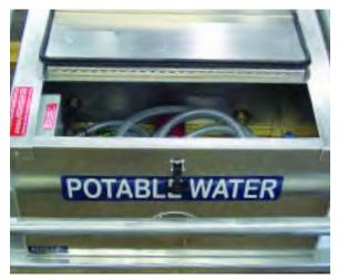
Pump & components in insulated, sealed compartment
