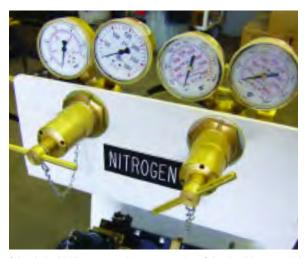
3-bottle Lo-Hi Nitrogen regulator mounted on 3-bottle tilting cart with nitrogen booster
