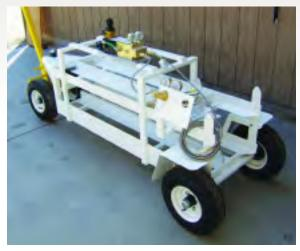
4-bottle oxygen regulator mounted on cart with oxygen booster
