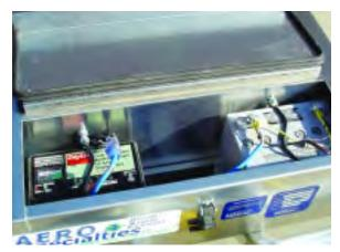
Battery & charger in insulated, sealed compartment
